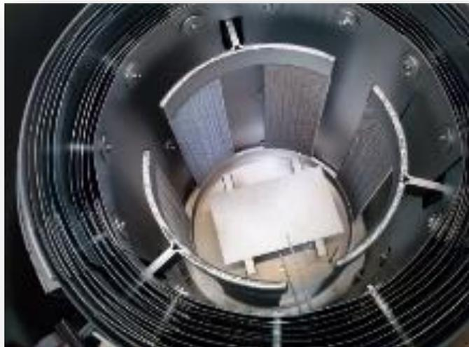
$T_{\max} = 2000^{\circ}\text{C}$  (W elements)
