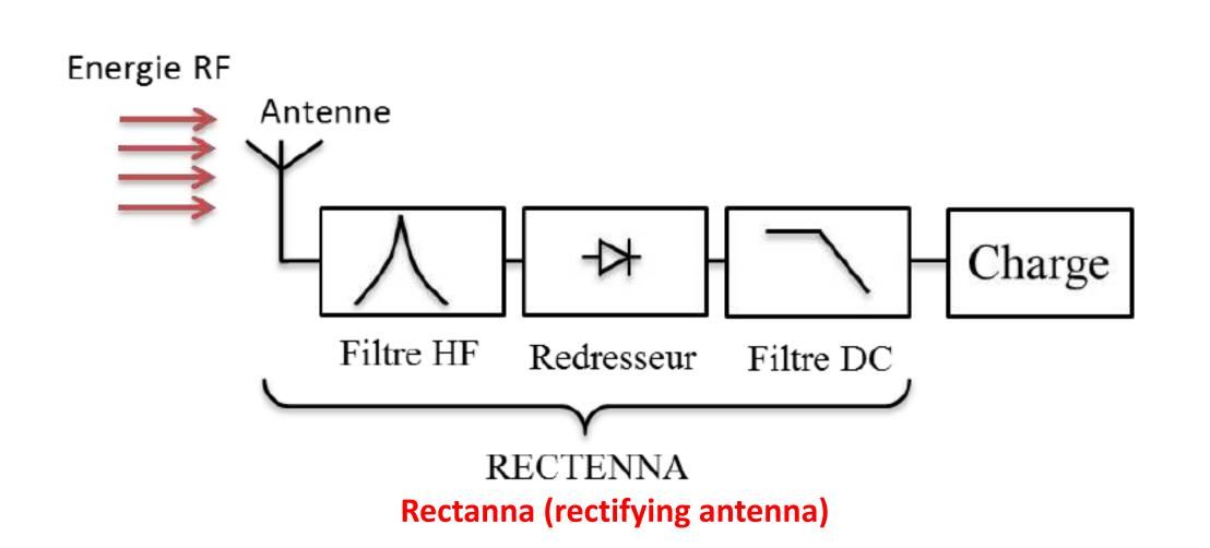
The schottky diode is the main part of the Rectenna in order to rectify the input AC signal and deliver the DC output signal required to power the main circuit.
