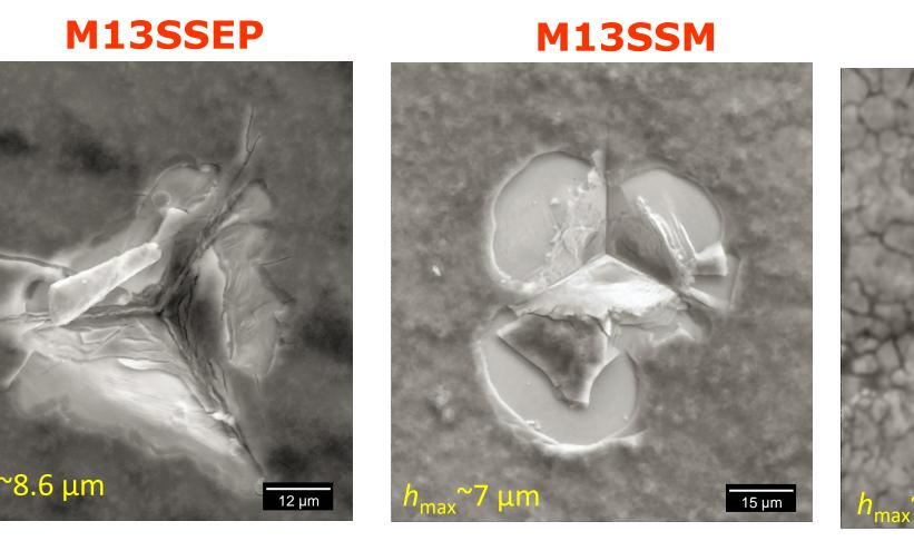
Indents from tests at higher penetration depths showing chipping due to coating decohesion
