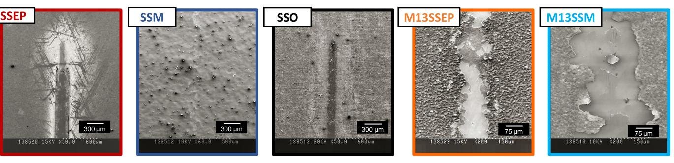
Substrate is reached during wear tests in NaCl solution for M13SSEP and
